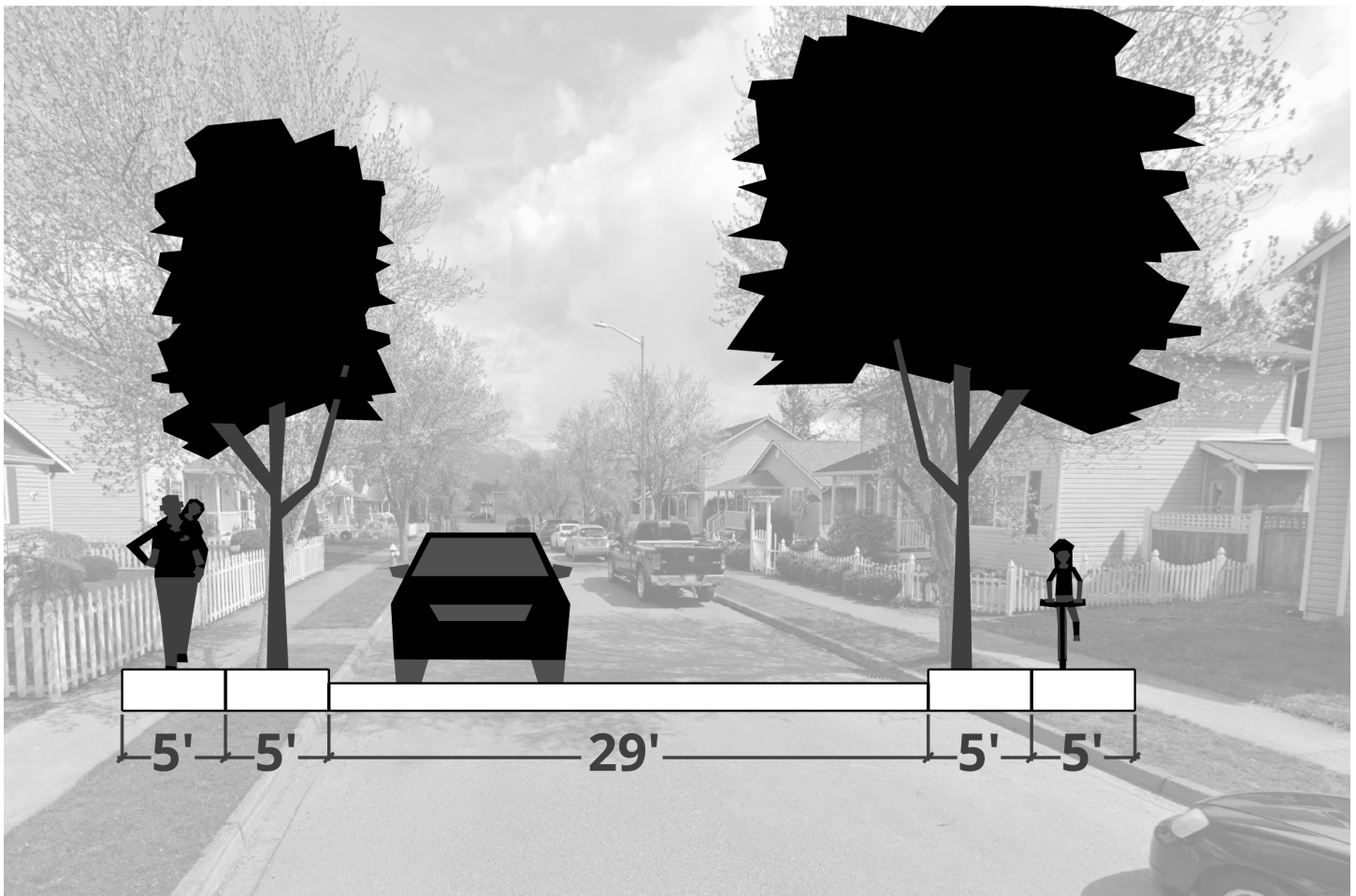
Figure 6 A street section from a newer subdivision located north off of Sultan Basin Road.
